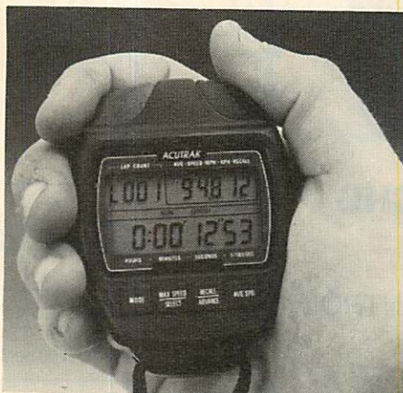
This shows the speed calculation result. On a track of 330 metres, with a lap time of 12.53 seconds, the vehicle being timed was travelling at almost 95 kilometres per hour.
