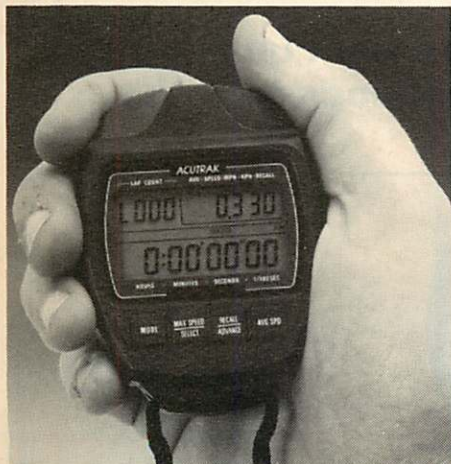
In Speed mode, the Acutrak can be programmed with the track length, to allow it to calculate speed. In this example, the track length is 330 metres.
