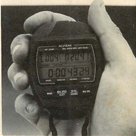
In chrono/lap mode, the Acutrak lap split function gives a reading of the actual time taken to do the lap, and using the recall function, five laps can be recalled.
